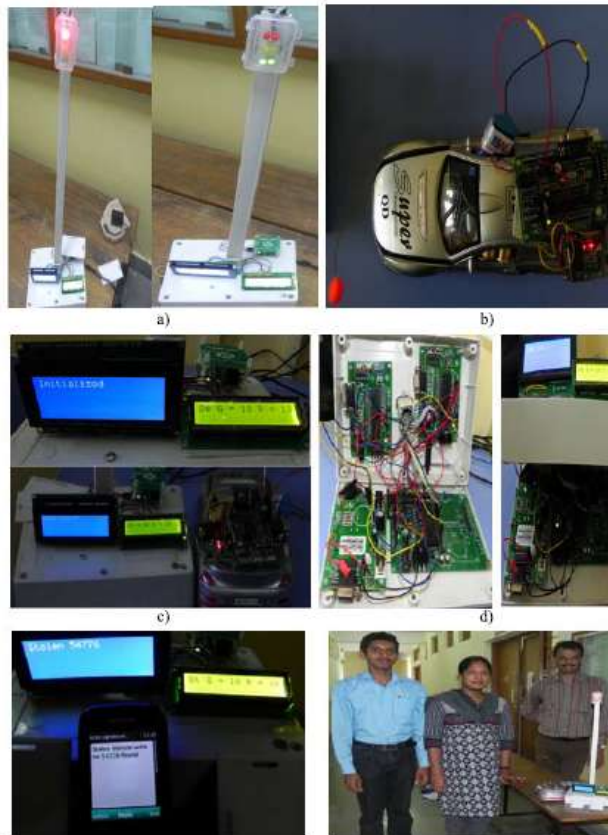
Fig. 5. Proposed model images transmitter and receiver. (a) Pole status at different condition. (b) Transmitter (ZigBee). (c) LCD display at receiver. (d) Detailed image of receiver. (e) When stolen vehicle is detected. (f) Working model. switch is pressed, it will transmit the signal. The signal contains unique id and security code. The transmitter contains PIC16F877A microcontroller and ZigBee module. The microcontroller sends the commands and data to the
